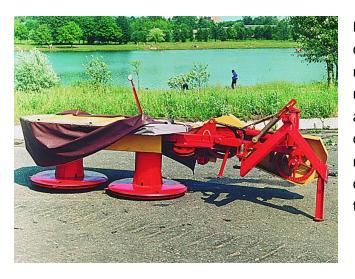
Rotor-type mowers L-501-01 is intended for mowing down grass and laying at the mowed surface. The mowing is accomplished as a result of rotation of two rotors with knives. To avoid damage when the hitting an obstacle the mower is equipped with damper device. Coupled with tractors of 0,9-1,4 type. The mower L-501D is an analogue of L-501-01, the difference is that it can be used for cutting slopes onthe-miter 45°.
